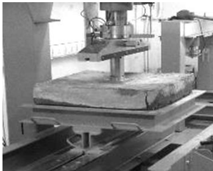
Flexure test of concrete slab
