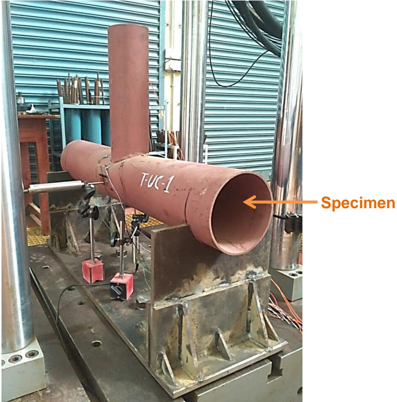
Flexure and fatigue tests of steel pipes
